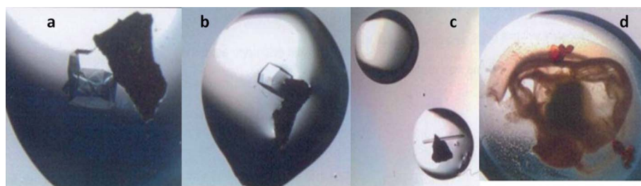
Fig. 7 Metastable crystallization drops containing generation 3 “functionalized” NPGs. (a and b) Large, single lysozyme crystals growing from NPG3 and NPG2 respectively. (c) A large single trypsin crystal growing from NPG4 and a clear control drop. (d) Haemoglobin crystals growing from NPG3, partially obscured by its characteristic precipitate.
